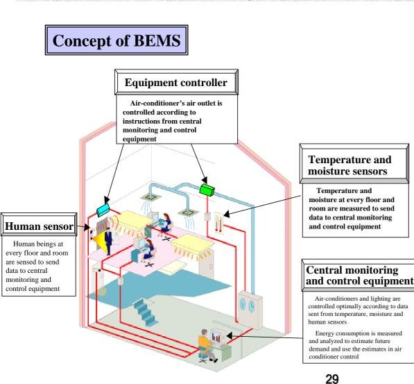
Promotion of dissemination of systems that support energy demand management in office buildings by making effective use of IT technology for realtime sensing of temperature and other room conditions in office buildings to permit optimum operation of lighting, air-conditioners and other equipment
