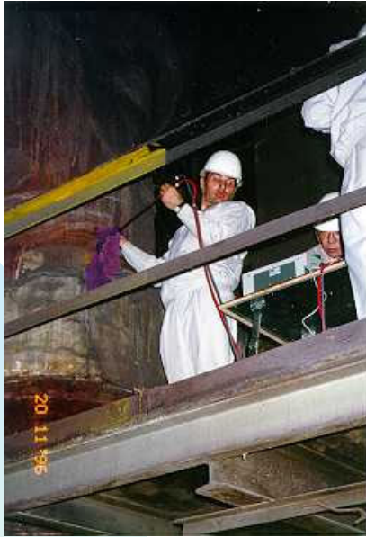
Steel works (flue gas rate measurement)
