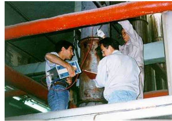
Textile factory audit (Dryer exhaust gas rate measurement)
