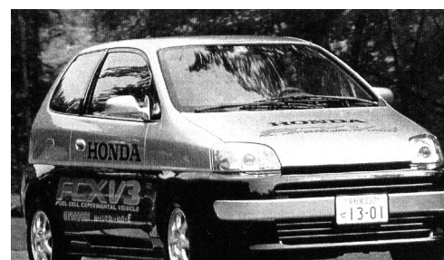
Source: Honda A fuel cell automobile, test driving on public road
