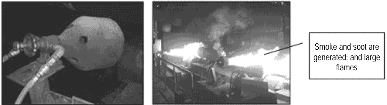
Fig. 16: Heavy oil burner and their burning state
