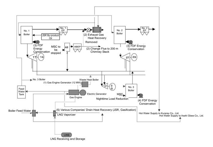
Planned Energy Conservation due to Recovery of Hot Water Heat from Various Industrial Complex Companies, Gas Cogeneration, and Other Measures.
