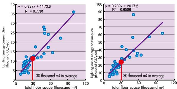
"Heat source + heat transfer energy" and "lighting energy" have high correlation with the total floor space.
