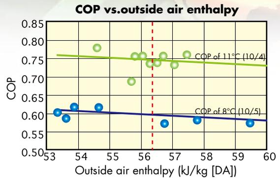
When the hot water outlet temperature is changed from 55°C to 45°C during early winter, the average gas consumption of the chilled/hot water generator decreased from 47.0 to 42.5 m<sup>3</sup>/h, and resulted in **10%** energy conservation.
