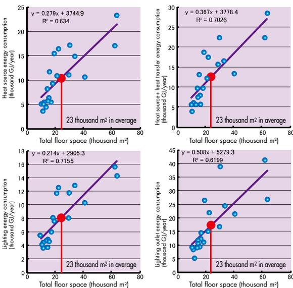
As to the correlation with the total floor space, “heat source + heat transfer energy” has higher correlation than the “heat source energy” .
