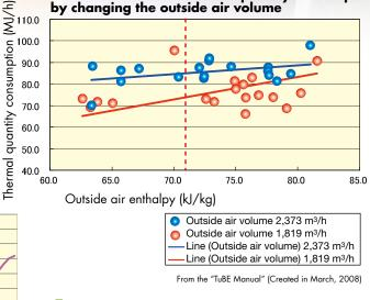
Convert the verification results to below 1,000 ppm. Increase outsideair volume to 2,130 m<sup>3</sup>/h; (1100 - 400)/(1000 - 400) = 1.17 times. Chilled water thermal quantity will be reduced by 8.5 MJ/h; (10 MJ/h)/1.17 = 8.5 MJ/h.
