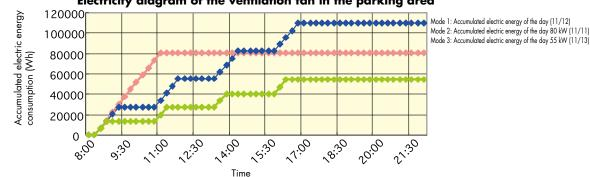
Electricity diagram of the ventilation fan in the parking area
