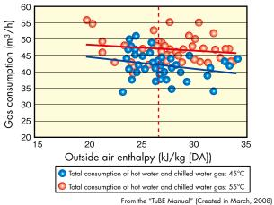
When the hot water outlet temperature is changed from 55°C to 45°C during early winter, the average gas consumption of the chilled/hot water generator decreased from 47.0 to 42.5 m<sup>3</sup>/h, and resulted in 10% energy conservation.
