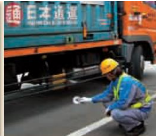
Check of black smoke using a black smoke chart
