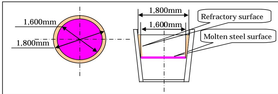
Fig. III-2-4 Heat radiation from the 25t-ladle
