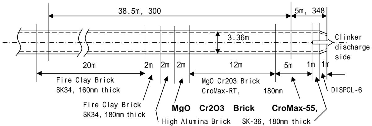
Figure IV-2-2 Refractory arrangement in the kiln section
