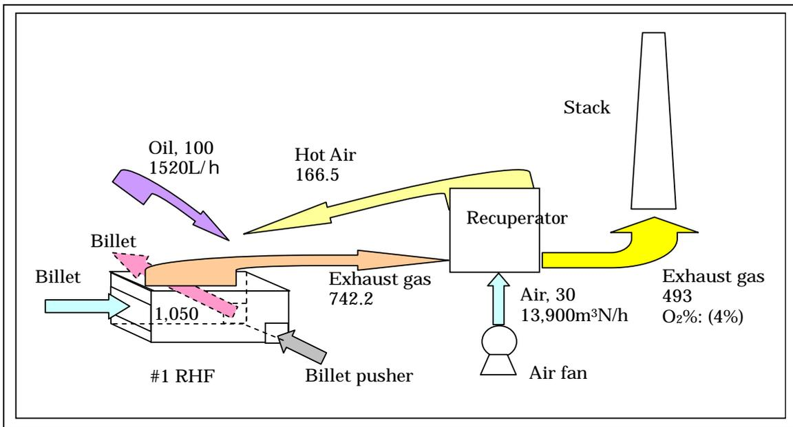
Fig. III-2-2 Data concerning combustion in the heating-furnace #1
