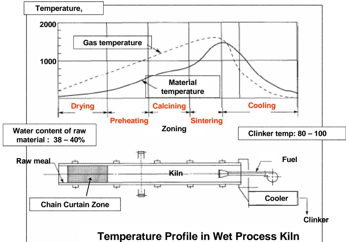
Figure IV-2-1 Typical temperature profile inside a wet-process rotary kiln
