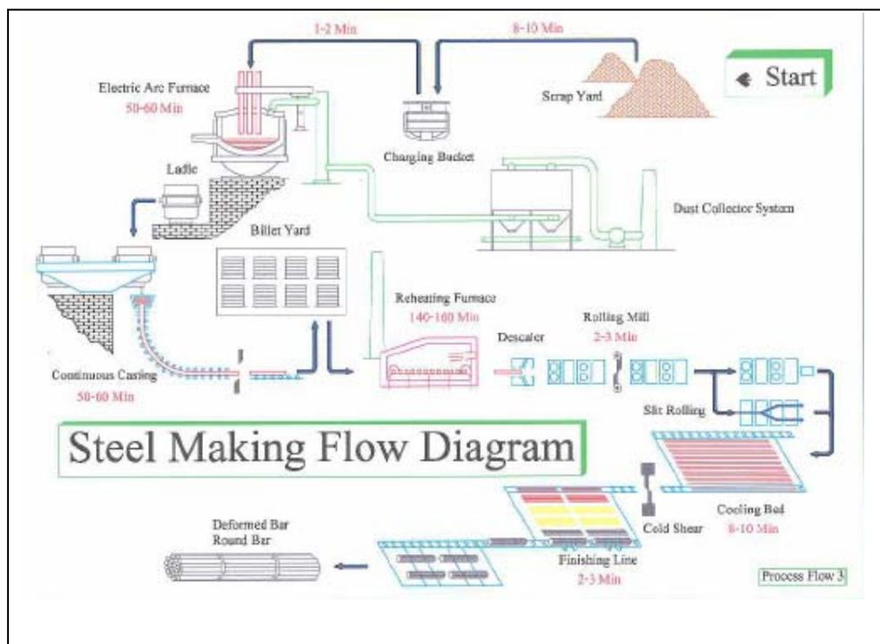
Fig. III-2-1 Concrete reinforcing bar manufacturing process
