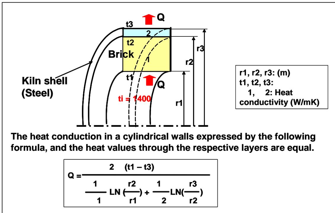
Figure IV-2-3 Heat transfer calculation for kiln refractory
