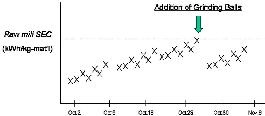
Fig. II-2-1 Management of grinding SEC in a ball mill
