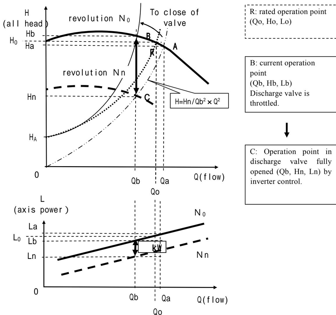
Fig. III-2-5 Electric energy saving by changing pump rotational speed
