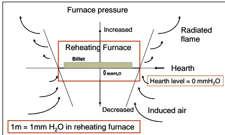
Fig. III-2-3 Relation between furnace pressure, air inflow and gas
