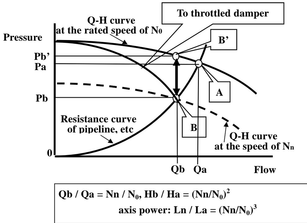
Figure IV-2-4 Energy saving effect through inverter installation illustrated on the performance curve of fans and blowers
