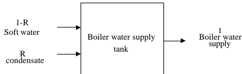
There are two types of condensate, clean and dirty. The clean condensate is a condensate generated from the steam used for indirect heating. It does not contact directly with process fluid, and becomes an object of recovery into the boiler water tank.
