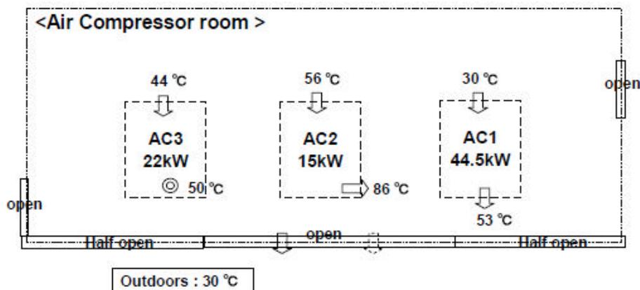
Calculation for compressor power reduction rate
