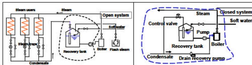
Figure 9-5 Condensate Recovery System (open-type vs closed-type)
