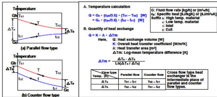
Figure 9-4 Countercurrent-type Heat Exchanger
