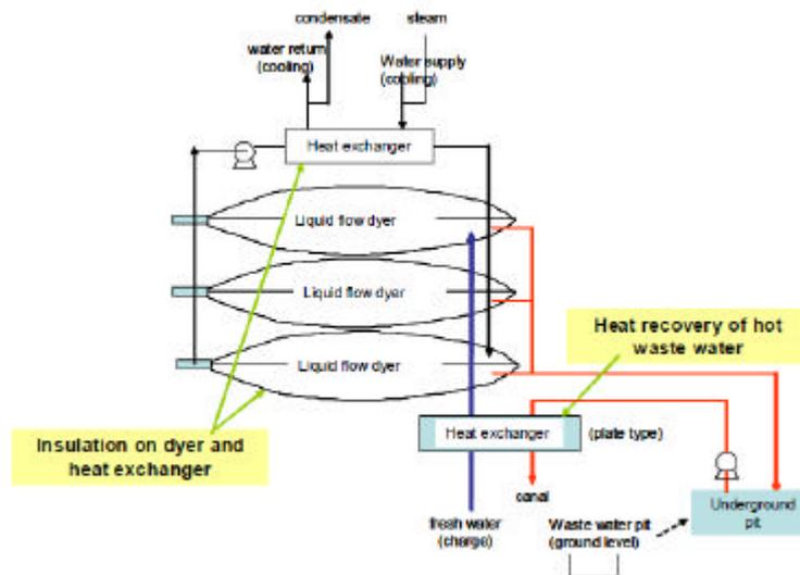
The dyer operates by batch of two cycles per day with eleven hours per cycle. Production capacity of cloth per cycle is 800kg. 10kg of dye liquor or washing water is used per cloth of 1kg (called bath ratio 10). Dyeing, neutralization and washing are repeated during one cycle according to the recipe in Figure 9-2.
