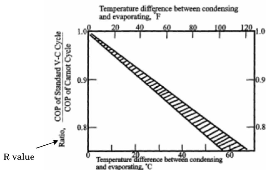
R value (ratio of COP of the standard cycle to COP of the Carnot's reversible cycle) was calculated based on the following figure. Refrigeration compressor efficiency was assumed to be 80%.
