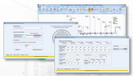
The heat exchanger unit operation incorporates an advanced geometry design algorithm that provides user-specified design constraints and options based on known limitations for the new or retrofitted exchanger.
