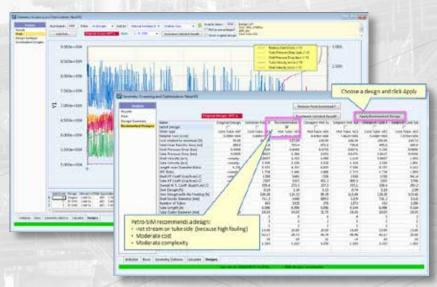
Potential design options are assessed based on the supplied pressure drop and velocity criteria, and then ranked based on relative cost criteria.
