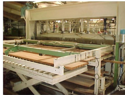
Figure 2 : sticking composite parts by High Frequency process
